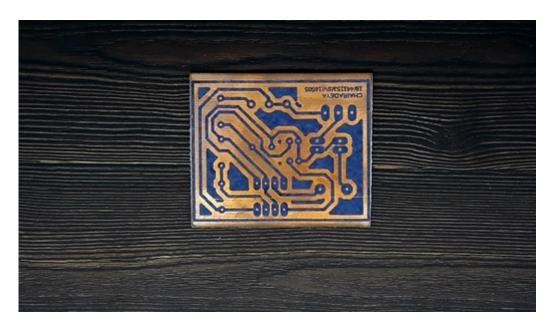
After that, we will etch the PCB with ferric chloric ( $FeCl_3$ ) and water ( $H_2O$ ) solution. After the dissolution process is complete the PCB board is cleaned with water so that the PCB path can be seen
