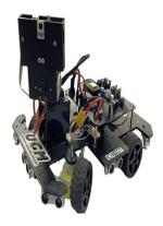
Implementation of Steering Based Path Following on Prototype Self-driving Car Robot using Pixy2 Vision
