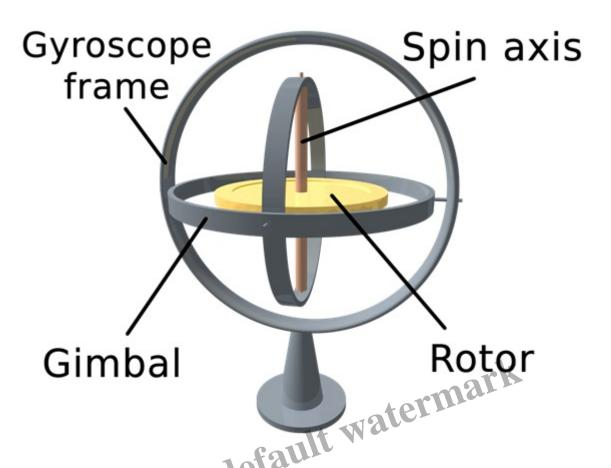
Gyroscope is a device for measuring or maintaining orientation, with the principle of angular
