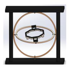
Test Bench Gimbals Rig for Quadcopter CAD Design
