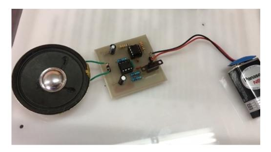
This circuit works by using a siren that has 2 different tones and alternates with double IC NE 555. Each IC is set as a different tone generator, IC 1 is lower and IC 2 is higher. IC 1 produces lower noise by adding smaller resistors than resistors on the larger IC 2. Then the tone is connected via pin 5 IC NE 555. The way of combining these 2 notes is work by superimposing the low notes to the higher notes. While the time interval that occurs is regulated by a capacitor.
