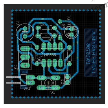
In here, I using 0,8 mm width rout and 0,8 mm drill. We can also check the 3D model of our PCB's project using AUTODESK Fusion 360.
