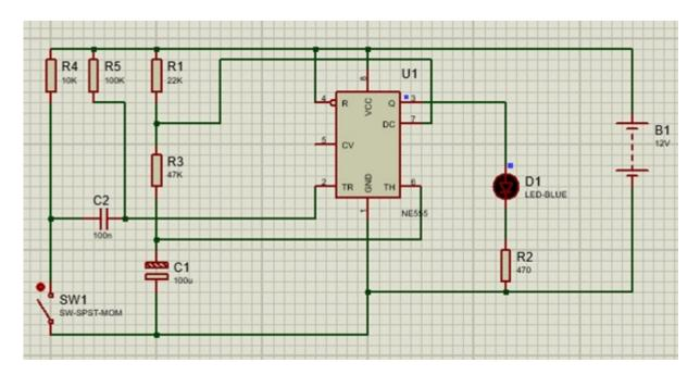
On that picture, when the press button (SW1) didn't connected, the LED wouldn't light up.
