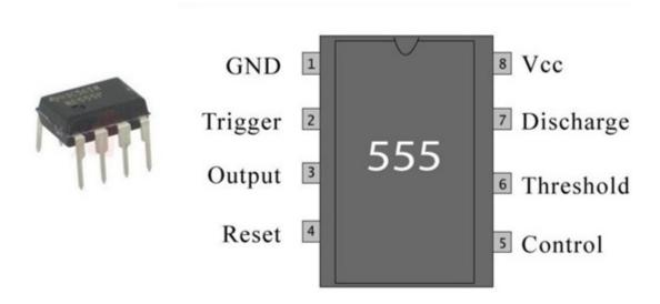
Here is picture of IC NE555. Its got 8 pin/ dip that have their own function.
