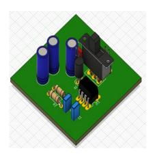
Machine Gun Sound Circuit Using IC NE555
