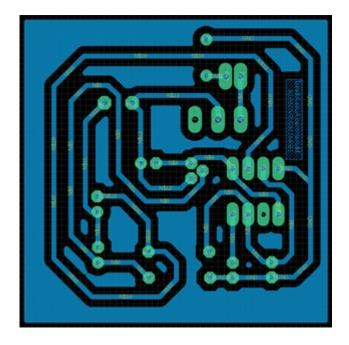
After we had made the schematic, we switch to Board. The size of the board I had made is 5cm x 5cm. The route and the pads I used is large to prevent mistakes when we are soldering the components to the PCB. This could cause the failing of the circuit and we have to try again.
